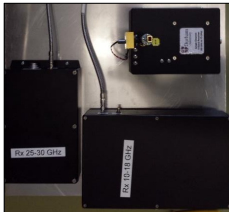
Figure 3-3 RF heads for all frequency bands at the receiver side
