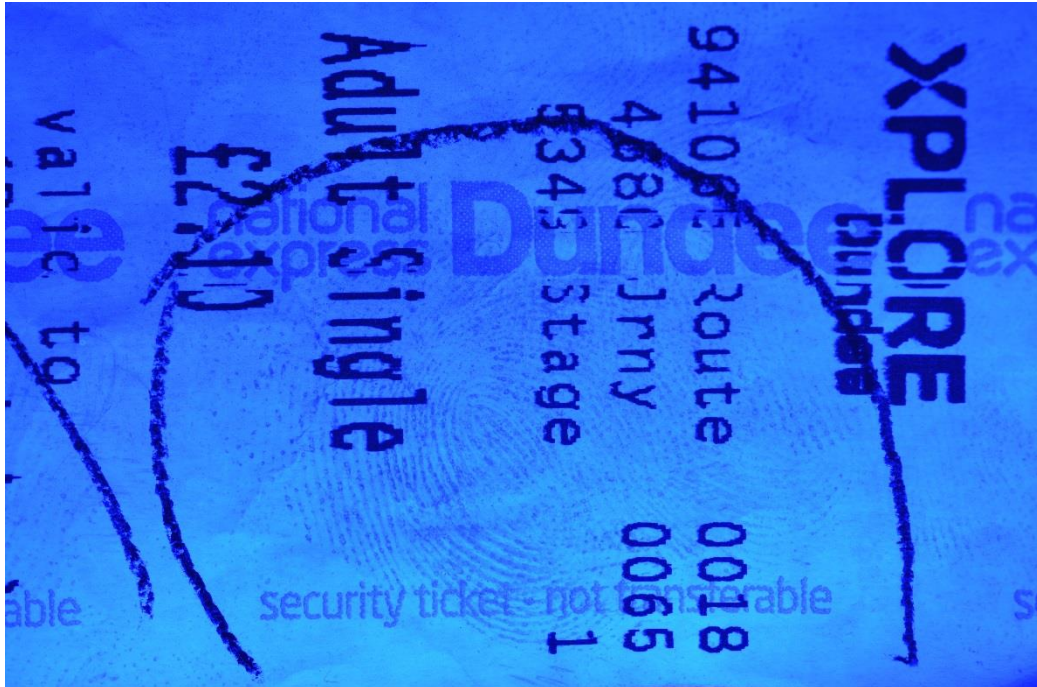
Figure 4 – Latent fingerprint developed with UV-A and viewed with a UV filter
