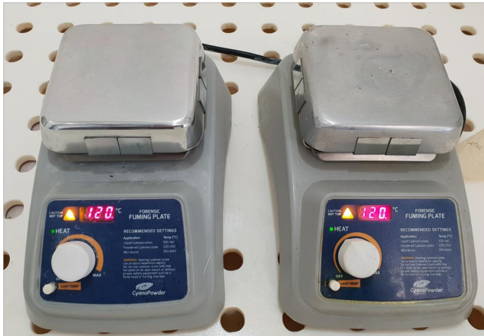
FIG. 2 – The two hot plates in the CA fuming chamber used during co-fuming.
