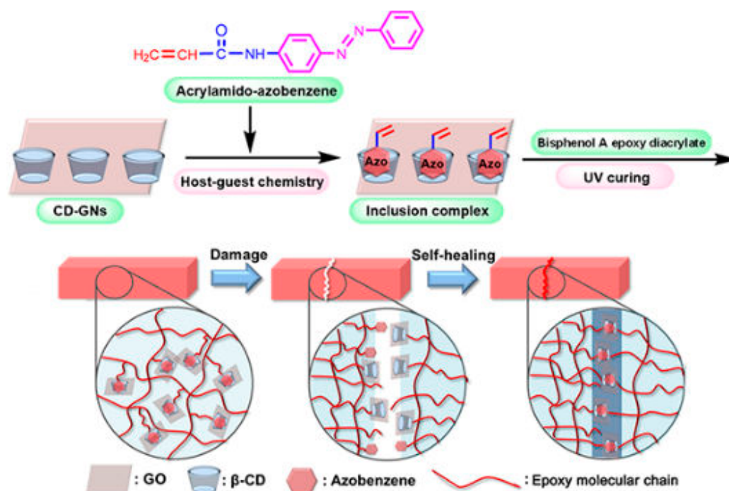
Figure 12. Schematic illustration of the self-healing mechanism of epoxy composite films. (Reprinted with permission from [89]. Copyright American Chemical Society, 2018).
