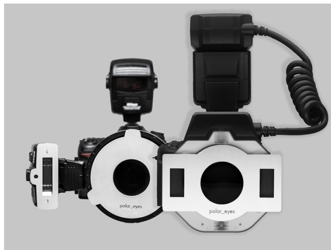
FIGURE 5 The use of cross polarization presents a convenient method to record the appearance of teeth without surface reflections (gloss) to ensure accurate color measurement. The most straightforward approach to achieving adequate cross polarization is with the use of a ring flash, paired with the appropriate cross polarization filter
