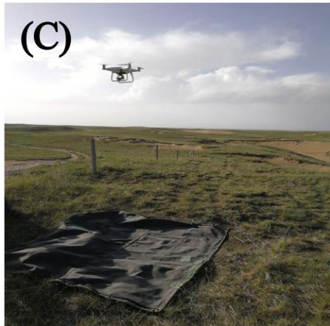
Figure 2. Pictures of the field UAV flying and measurement of the GCPs. (A) The customized GCPs sign is made of cloth material. The middle hole was used for the wooden stake to pass through, and the four corner holes were used to fix the sign. (B) The coordinate measurement of the GCPs. (C) Picture of the UAV performing a flight mission.
