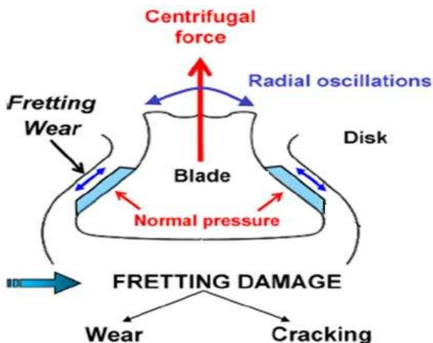
Fig. 2 Schematic diagram of fretting wear between blade mortise and turbine disc under working conditions
