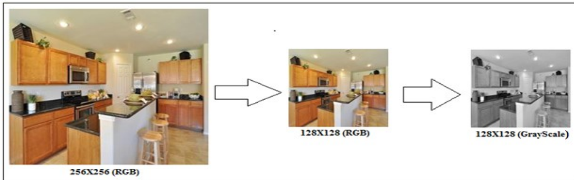
Fig. 4. The conversion of 256X256 (RGB) image to 128X128 (Grayscale) image
