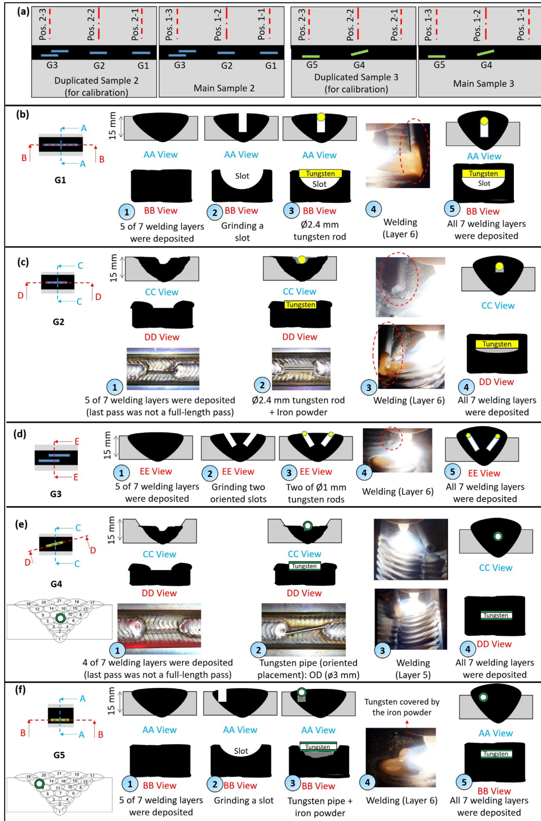
Figure 5. Position (a) and procedure (b-f) of the intentionally-embedded defects (G1-G5)
