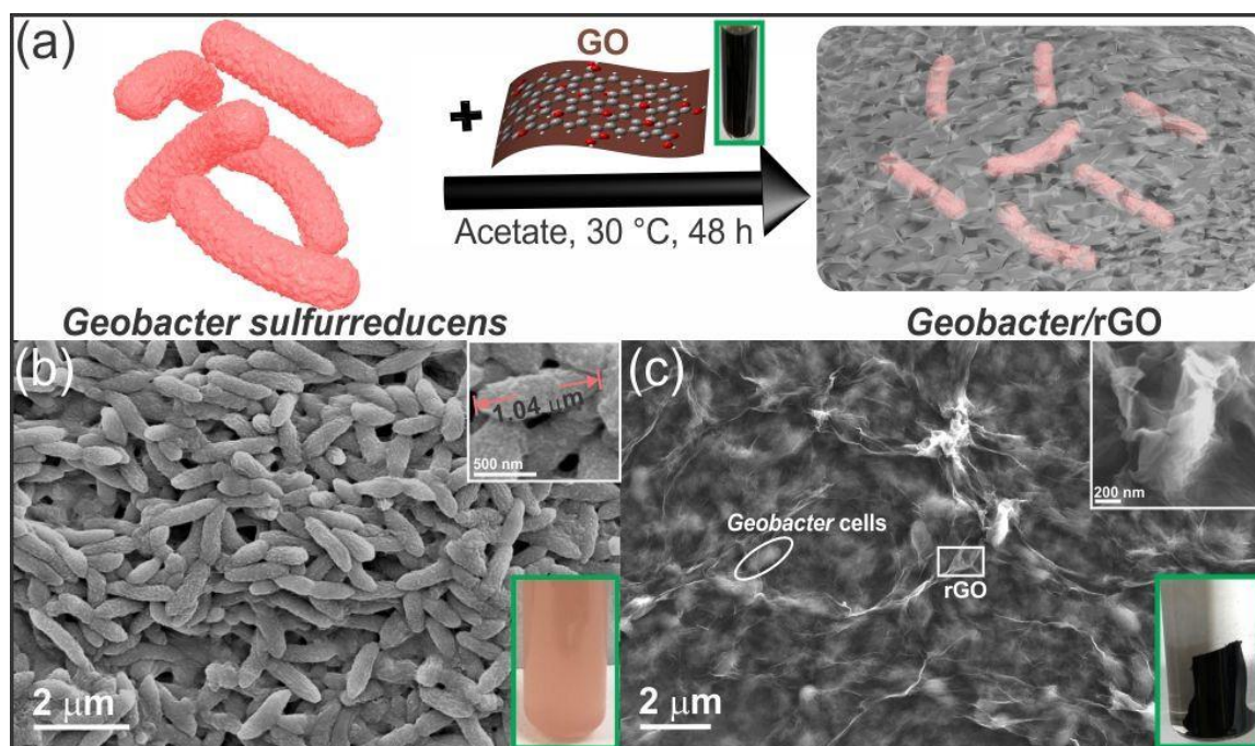
Figure 1. Schematic illustration and morphological characterization. (a) Schematic illustration for the reduction of graphene oxide (GO) by G. sulfurreducens (conditions: 30 °C, anaerobic, pH 7).
