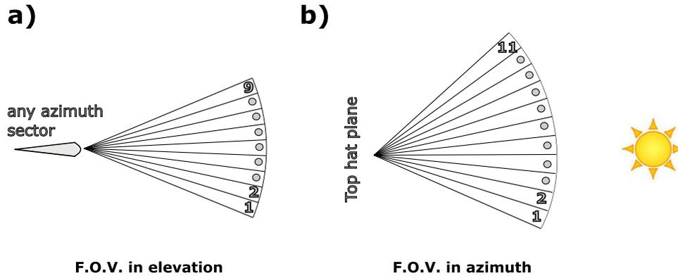
**Figure 2.** Field of view (FOV) of the SWA-PAS instrument: (a) The elevation FOV covers angles from  $-22.5^\circ$  to  $+22.5^\circ$  with respect to the Sunward direction through nine electrostatic sectors with a resolution of  $\sim 5^\circ$ . (b) The azimuth FOV covers angles from  $-24^\circ$  to  $+42^\circ$  with respect to the Sunward direction through 11 azimuth sectors (physical sectors of the instrument) with a resolution of  $\sim 6^\circ$ .
