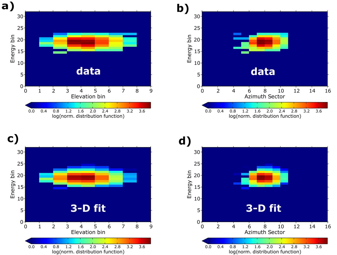
**Figure 10.** (a) The elevation-energy matrix and (b) the azimuth-energy matrix of the proton distribution function observed by *Helios 2* on day 67 of year 1976 at 22:32:33 UT. (c) The elevation-energy and (d) the azimuth-energy matrix of the 3D isotropic kappa distribution fit.
