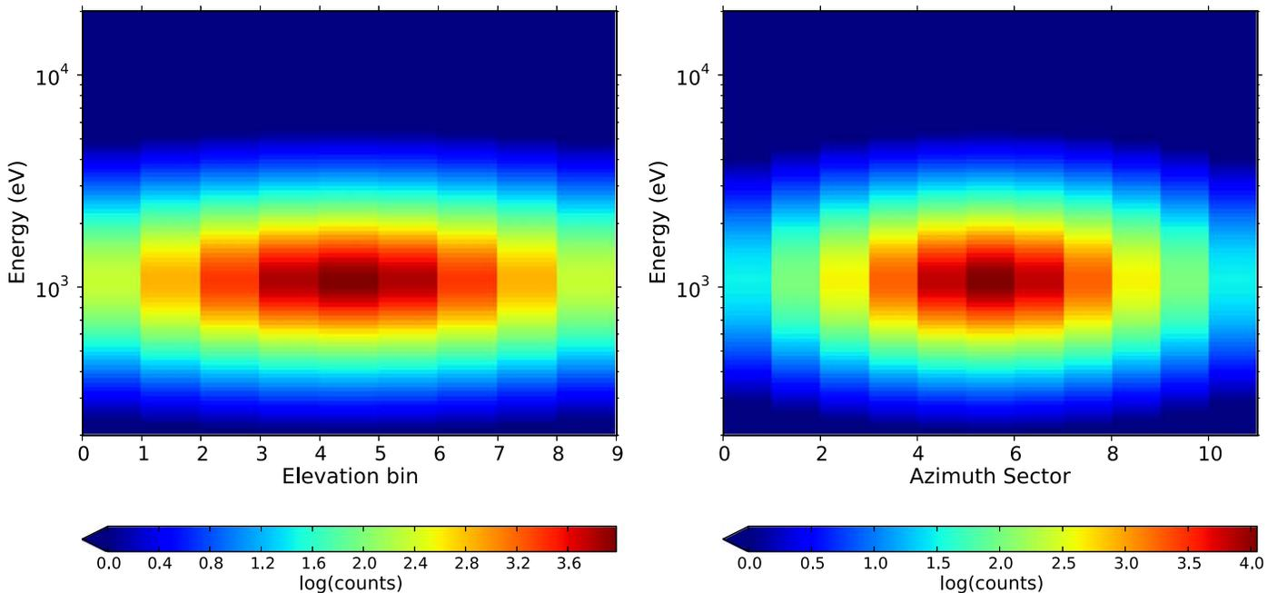
**Figure 3.** (Left) Elevation-energy matrix and (right) azimuth-energy matrix of SWA-PAS pseudo-observations for protons with bulk energy  $E_0 = 1$  keV, temperature  $T = 40$  eV, and a  $\kappa = 3$ .
