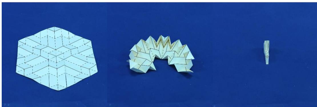
(b) Fig. 16 The regular hexagon pattern. (a) Improvement of the tessellation (no creases between red lines); (b) its folding sequence.
