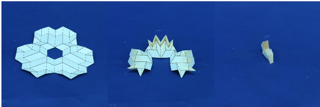
Fig. 15 Tessellation of the split pattern. (a) The pattern formed by six split patterns (no creases between red lines); (b) the card model of it.
