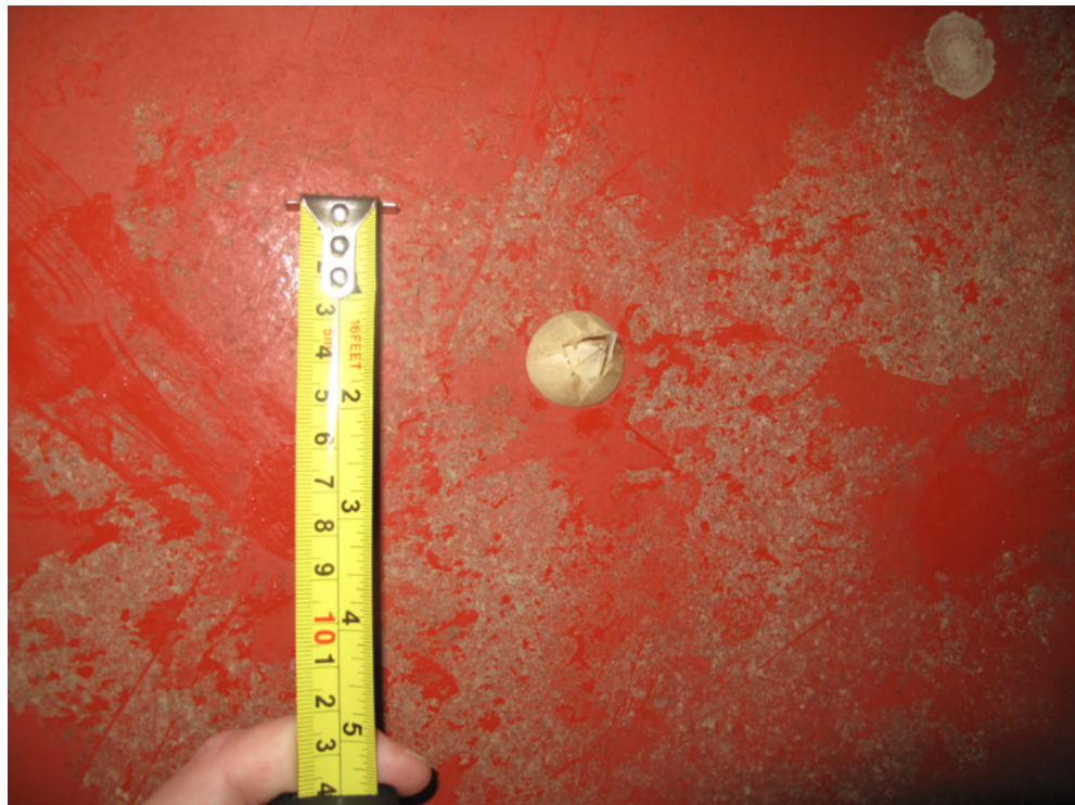
FIGURE 4: Barnacle biofouling on a deployed turbine blade showing a single, isolated barnacle. Image supplied by AHH.
