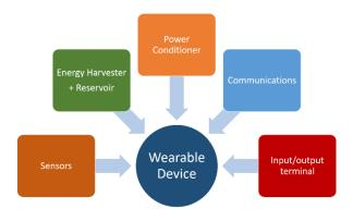
Figure 1. Building blocks of a wearable device.
