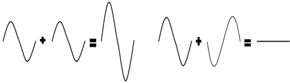
Figure 2.4: Constructive interference when wavelength is the same and waves are in phase, destructive interference when wavelength is the same and waves are out of phase
