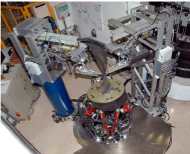
Figure 2.20: Photograph of SALSA with an aero-engine fan blade on the sample table(ref)
