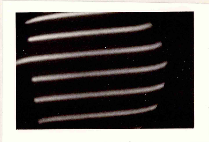
FIGURE 7.8b GRATICULE AT MAGNIFICATION OF FIGURE 7.9 One division equals 10 \mu\text{m} .
