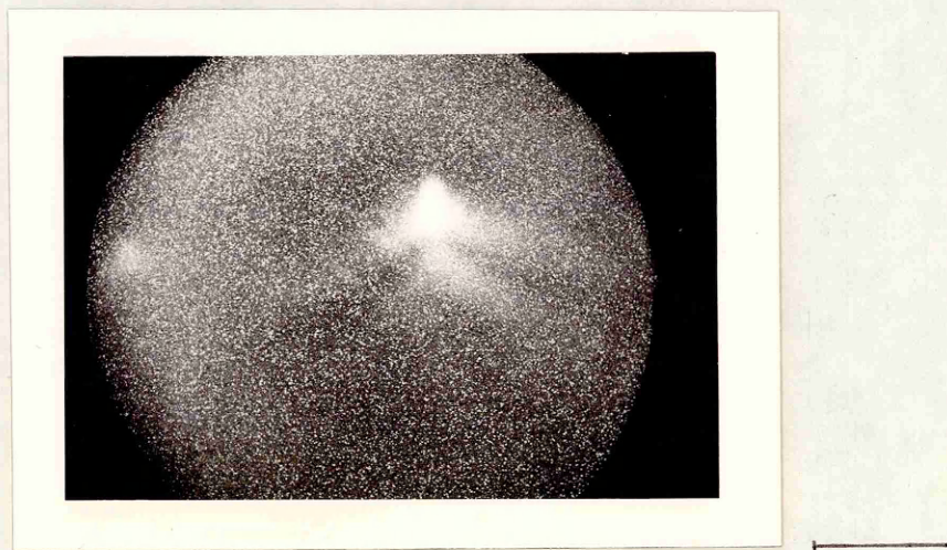
FIGURE 7.13b EL NEAR CONTACT 4 OF \text{Ga}_{1-x}\text{Al}_x\text{As} ( x = 0.52 ) SAMPLE, AT \approx 80 K WITH 150 V PULSES. Scale bar equals 10 \mu\text{m}
