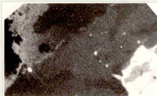
FIGURE 7.21b CATHODOLUMINESCENCE CONTRAST PHOTOGRAPH OF THE AREA OF \text{Ga}_{1-x}\text{Al}_x\text{As} ( x = 0.35 ) SHOWN IN FIGURE 7.19. Scale bar equals 100\ \mu\text{m} .
