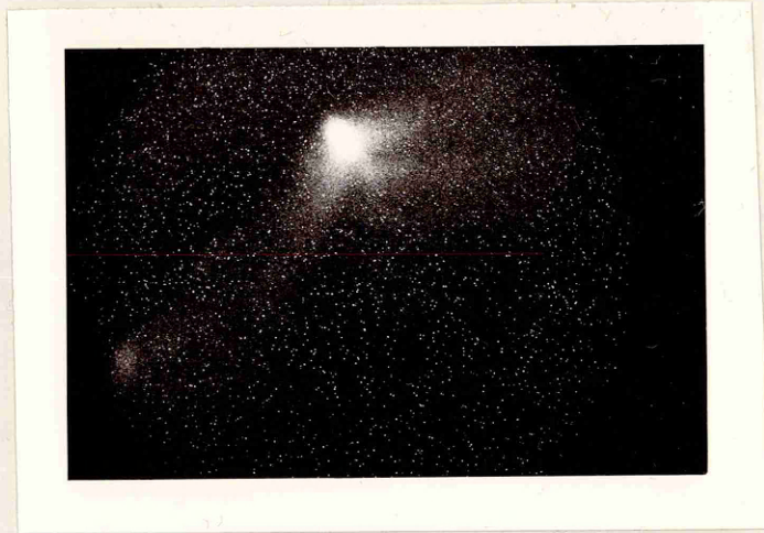
FIGURE 7.12a EL NEAR CONTACT 4 OF \text{Ga}_{1-x}\text{Al}_x\text{As} ( x = 0.52 ) SAMPLE, AT \approx 80 K WITH 90 V PULSES. Scale bar equals 10 \mu\text{m} .
