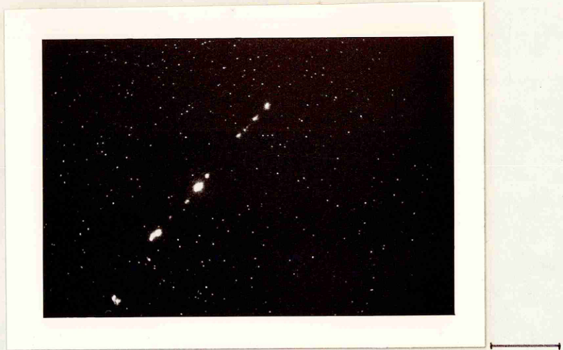
FIGURE 7.18a EL NEAR CONTACT 4 OF \text{Ga}_{1-x}\text{Al}_x\text{As} ( x = 0.35 ) WITH POLARITY 4^+ 1^- . Scale bar equals 100 \mu\text{m} .
