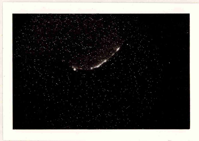
FIGURE 7.7b EL NEAR CONTACT 3 OF \text{Ga}_{1-x}\text{Al}_x\text{As} ( x = 0.52 ) SAMPLE One hundred x 0.1 second 72 volt pulses were used in this photograph. Sample at room temperature. Scale bar equals 50 \mu\text{m} .
