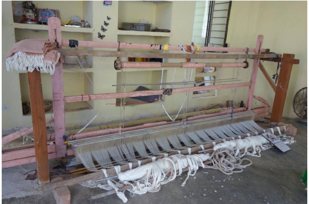
Figure P. Bedsheet loom, 90 inches in width (standard loom is 36 inches)
