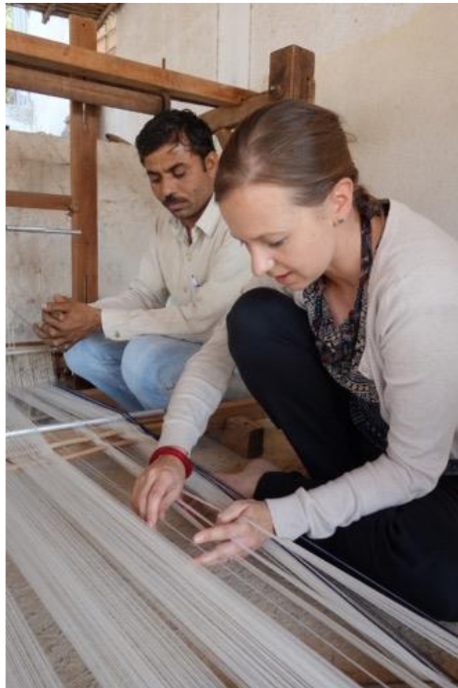
Figure 60. Counting the warp yarns to insert the extra vararch
