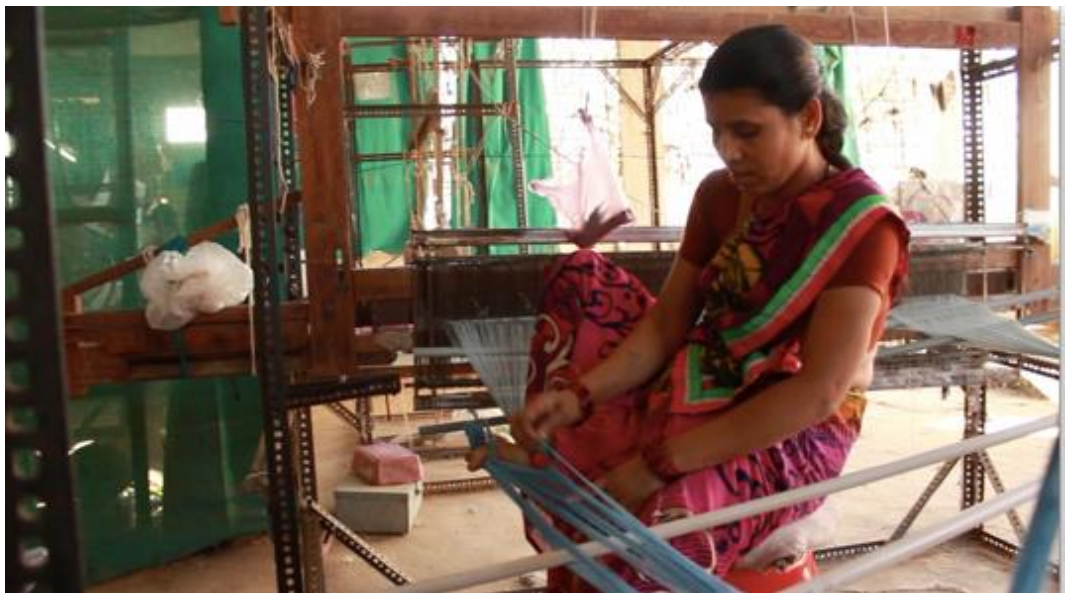
Figure 83. Joining the warp. Film still: Chayan Sonane
