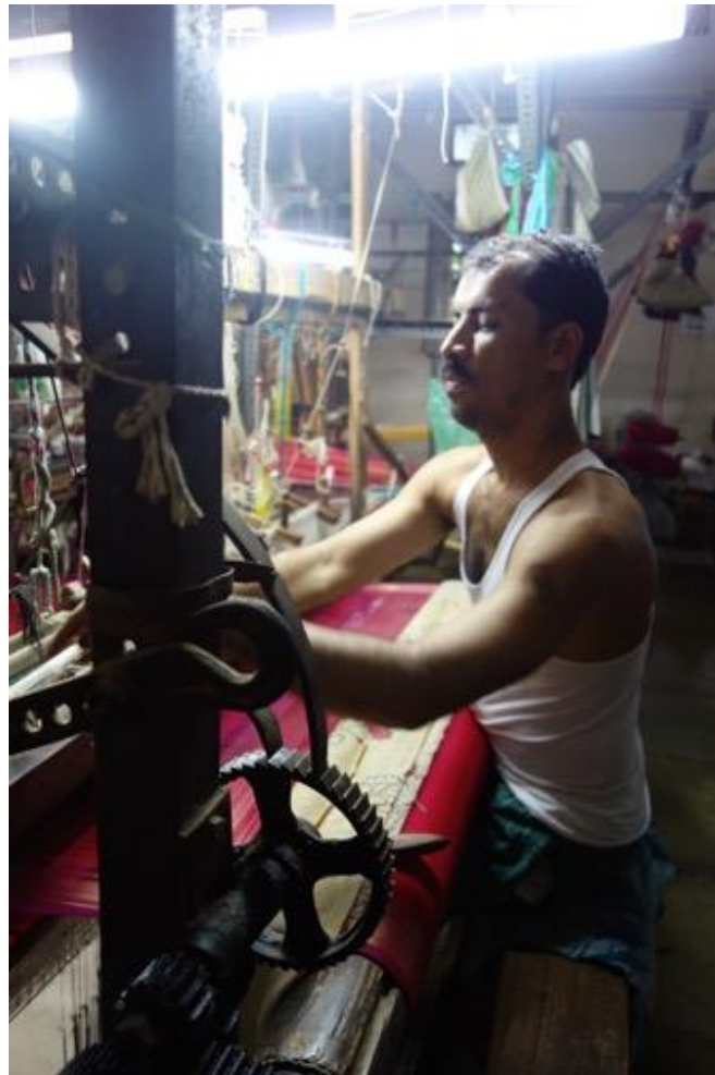
Figure 87. Take-up motion attachment
