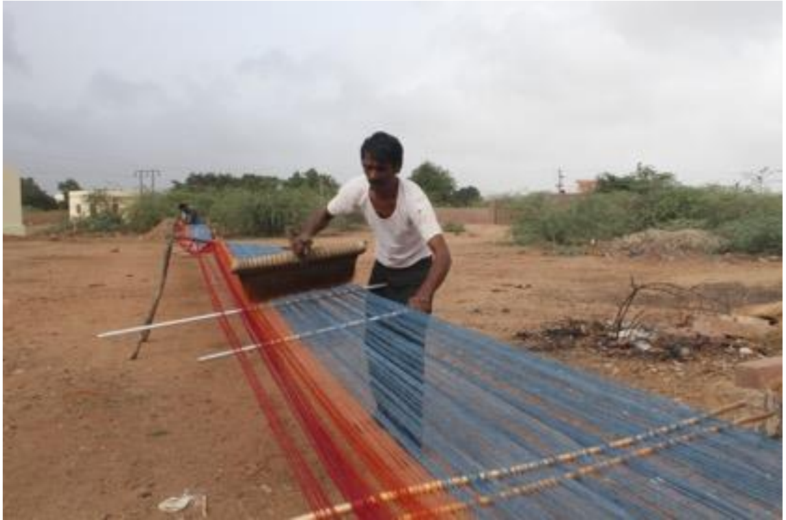
Figure 49. Spreading the starch evenly onto the warp using the kolori brush
