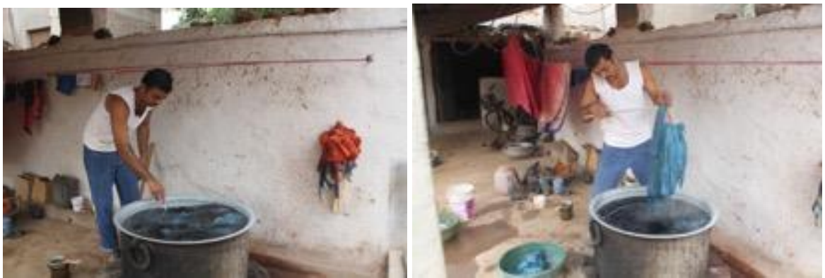
Figure 43. Dinesh Vishram Valji dyeing woollen yarns with acid dye. Photograph: Shradha Jain
