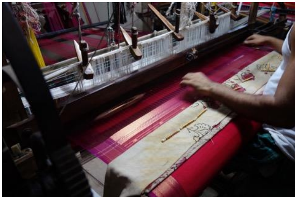
Figure 81. Loom with extra naka threads for extra drafting
