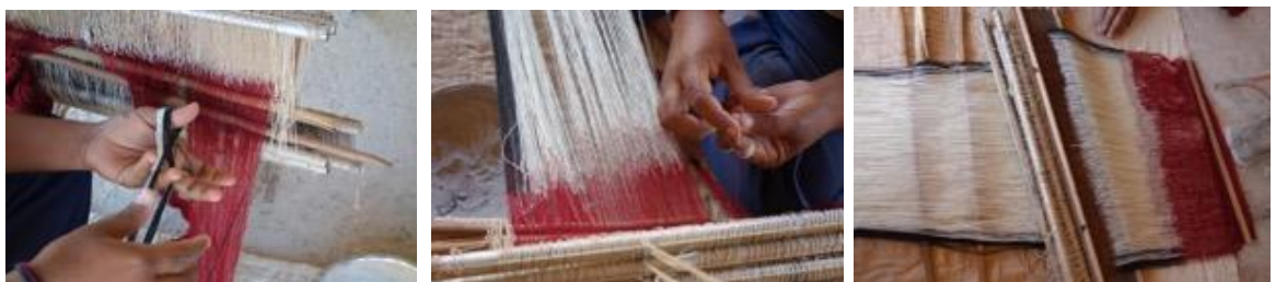
Figure 50. Joining the new warp to the ends of the existing warp
