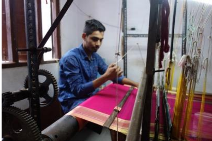
Figure 85. View of the dobby strings attached to the extra warp yarns
