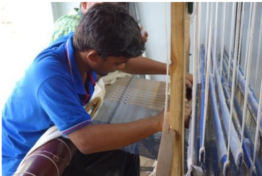
Figure 88. THS students Shahid and Dibya practising multi-treadling on different draft settings
