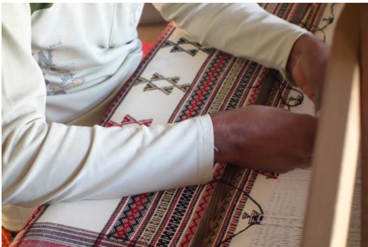
Figure 64. Inserting extra weft chomak , Ramparvekra village
