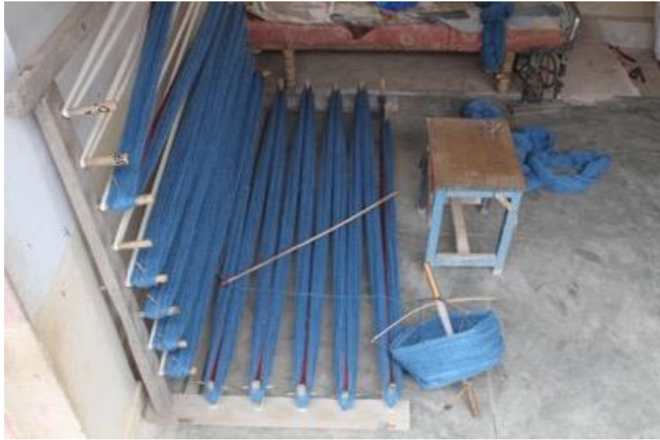
Figure 45. A 38 metres long warp for the bhediy -inspired blue and orange throws. Photograph: Shradha Jain
