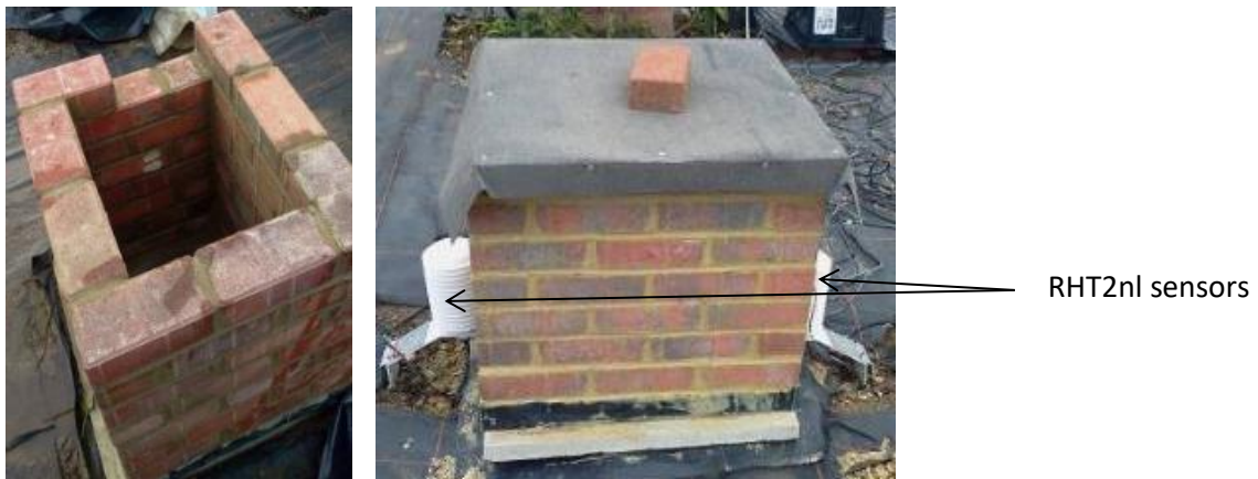
Figure 4 L-R: Bare model 'building' without roof (left) and with roof and screened RHT2nl sensors in situ (right)
