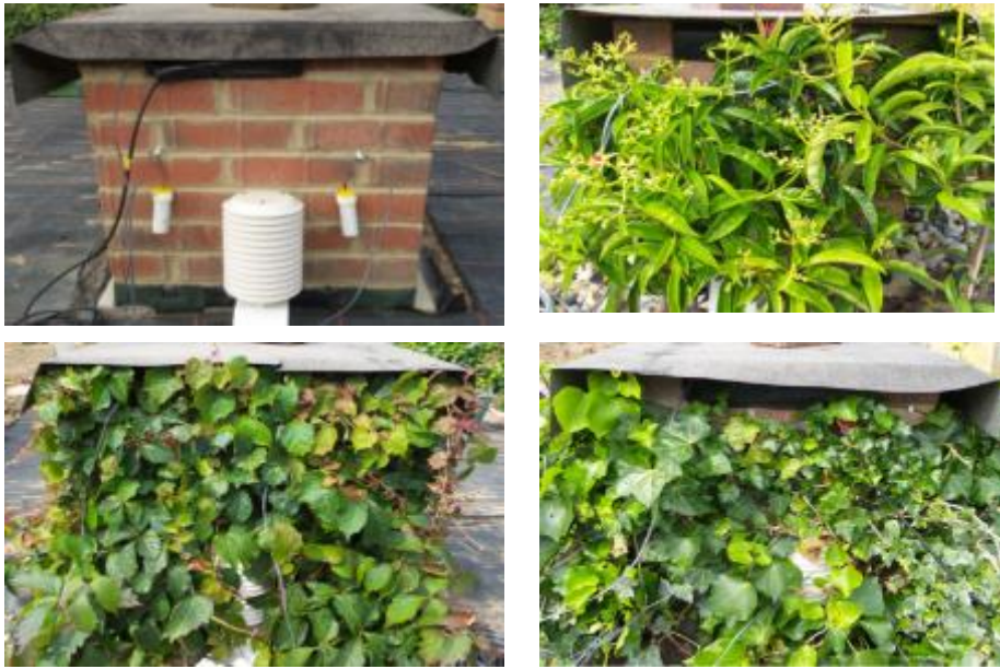
Figure 6 Top left to bottom right: Bare model 'building' and 'buildings' covered with Pileostegia viburnoides , Parthenocissus tricuspidata and Hedera helix , with roof and sensors in situ : set up for summer 2015
