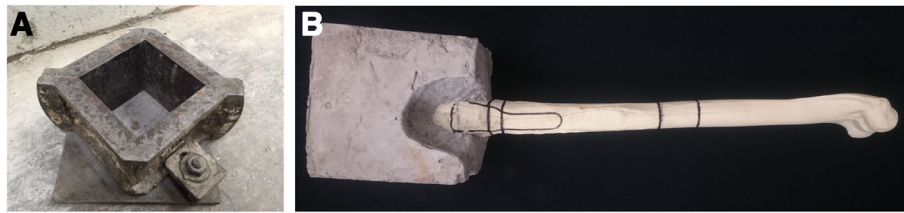
Fig. 2 Specimen preparation: Cubic mould (a) was filled with cement mix and humerus. After the block dried, humerus (b) was marked with positions of plate and cuts
