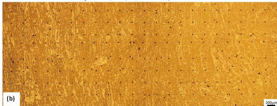
Fig. 3 The flow pattern development under a standard alignment (<25 μm) for (a) N = 1 turn and (b) N = 5 turns [18]
