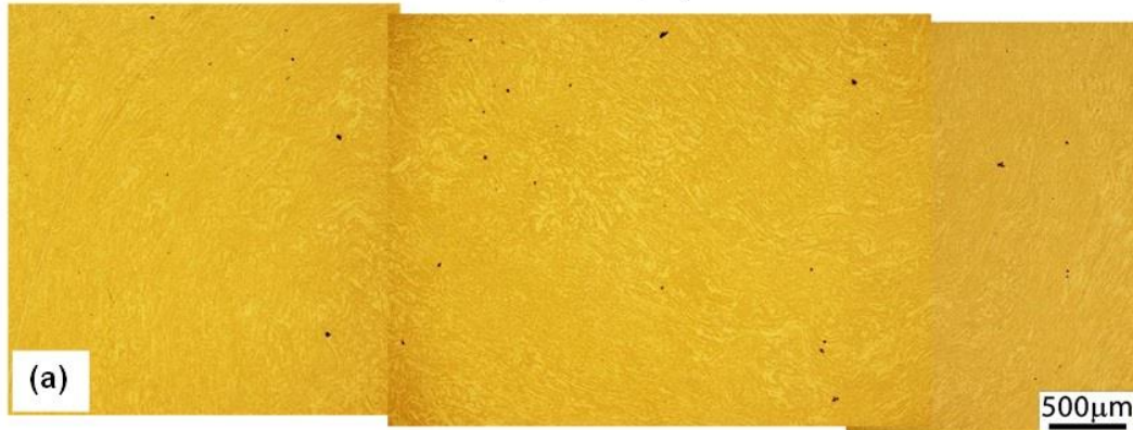
Rough anvil, misalignment of 100 \mu\text{m} , N = 1, top surface
