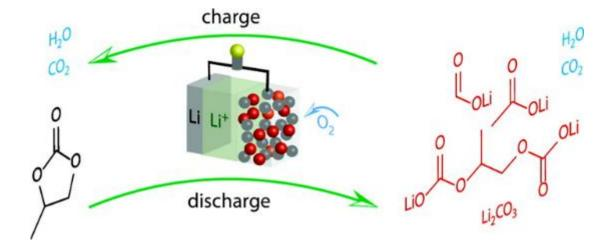
**Figure 12.** Graphical representation of charge –discharge of Li-O<sub>2</sub> cell with 1 M LiPF<sub>6</sub> in PC. Reproduced with permission from ref<sup>84</sup>. Copyright 2011 American Chemical Society.
