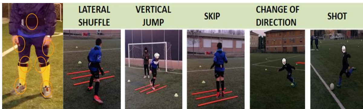
Figure 1 – Inertial sensors placement (left); pre-defined path for kinematic data acquisition (right)
