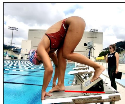
Figures 1a and 1b. Determining kick plate position based upon shin length measurement.
