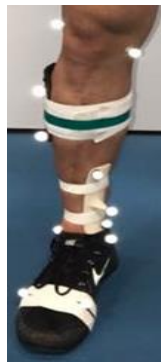
Figure 1: Anterior view of the 3D printed tibio marker plates used for dynamic movements.
