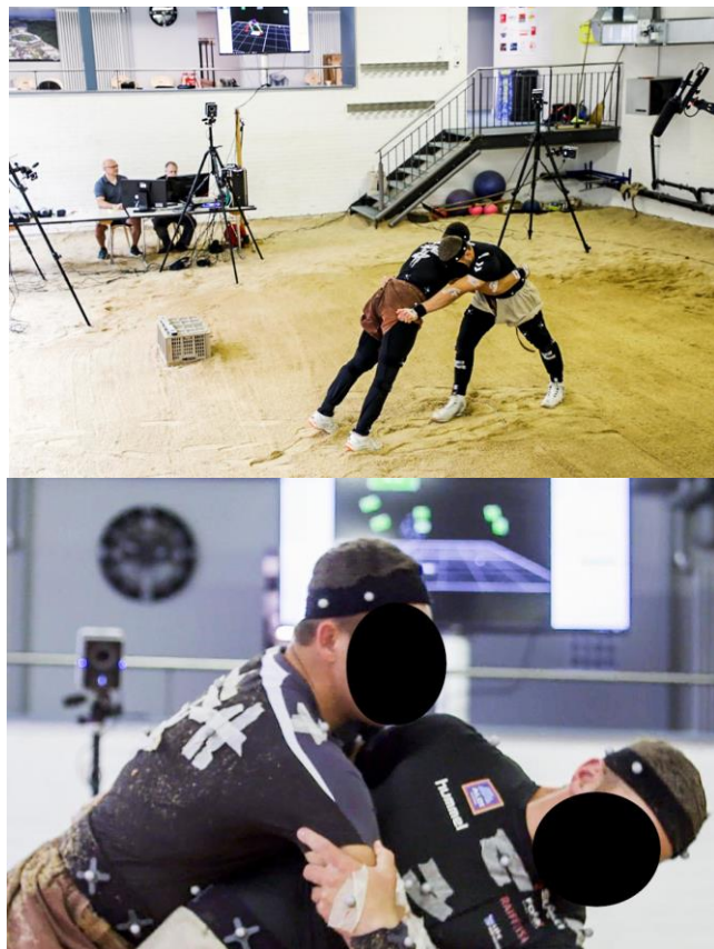
Figure 1: Measurement set-up (top) and optical markers on head, shoulder and upper body (bottom)
