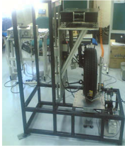
Fig. 2. The actual active suspension system.
