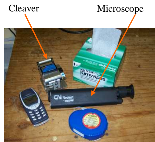
Figure 6.1 Miscellaneous fibre optic equipment.
