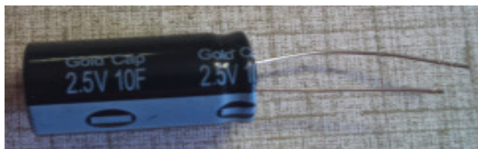
Figure 2.5. 10F, 2.5V supercapacitor.
