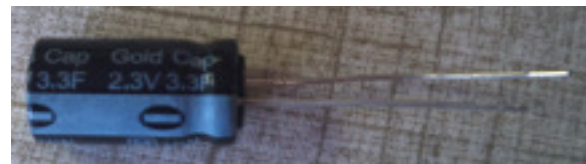
Figure 2.6. 3.3F, 2.5V supercapacitor.
