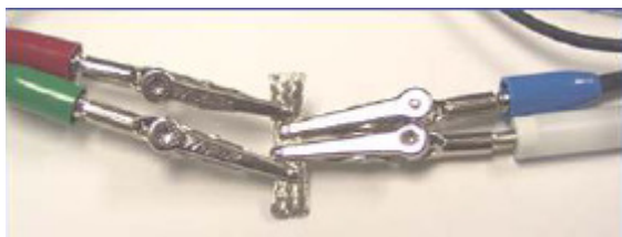
Figure 1.40. Cable setup during an EIS test.
