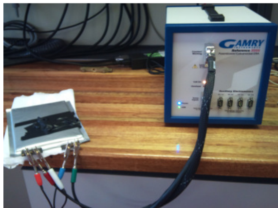
Figure 2.2. Gamry Impedance Analyser connected to a 20Ah pouch cell.
