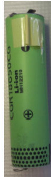
Figure 2.4 2Ah cylindrical cell.
