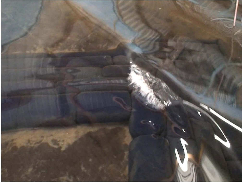
Figure 7.10 Image of wave breaking at the take-off area during model tests, the bag layout can be seen beneath the surface, as the wave peels left and right.
