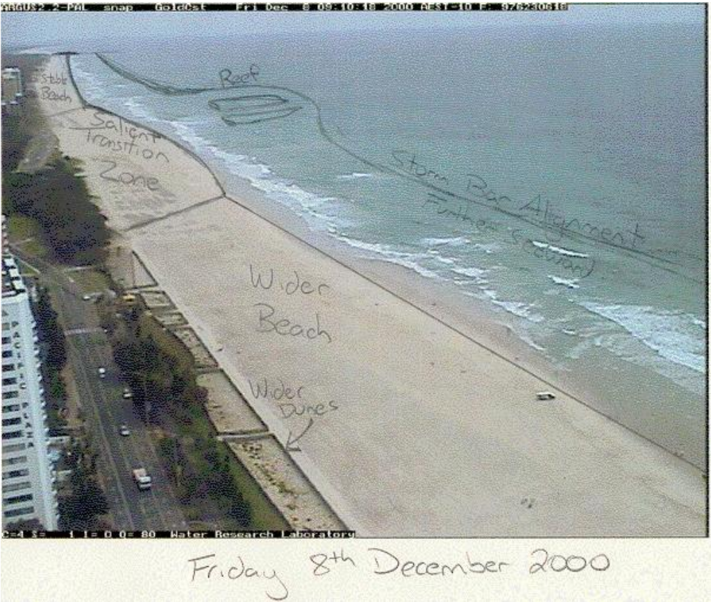
Figure 6.13 The Gold Coast multi-purpose reef was designed with a primary function of erosion control and secondarily to produce high-quality surfing waves. The notations are provided by John McGrath of the Gold Coast City Council (Mead et al. 2006).
