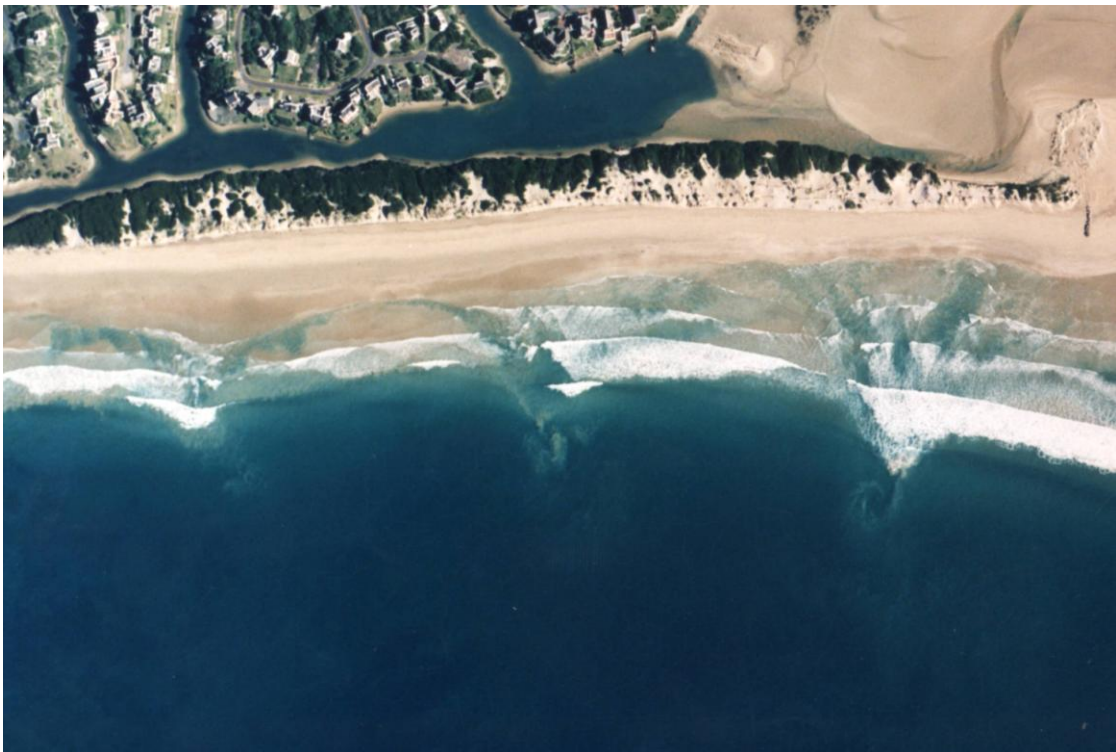
Figure 2.22 Aerial photograph of the northern end of St Francis Bay beach along the artificial sand spit/barrier dune, taken in July 1994. Several rip currents are clearly visible actively transporting suspended sediment offshore.
