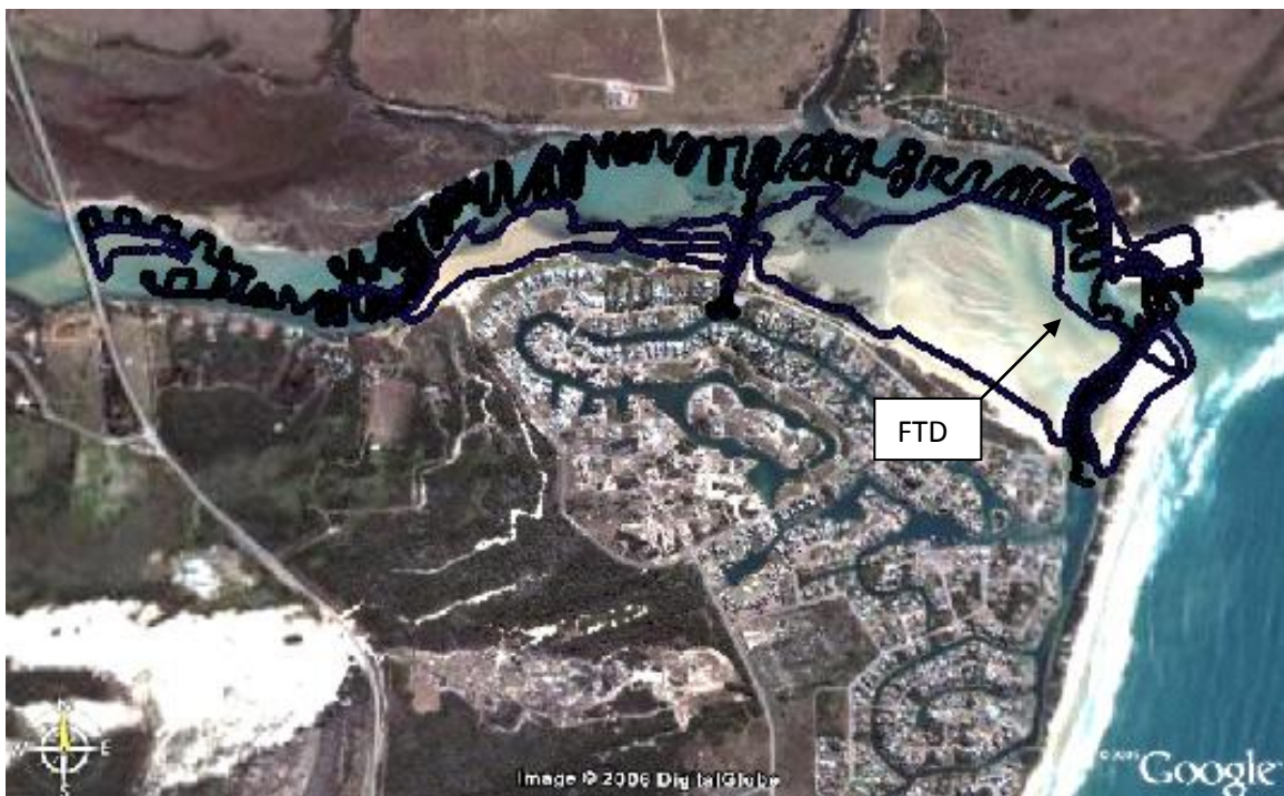
Figure 8.2 Satellite image of the lower Kromme Estuary with bathymetric survey lines indicated in black and inter-tidal survey coverage in dark blue. The large flood tidal delta (FTD) can be seen within the mouth.
