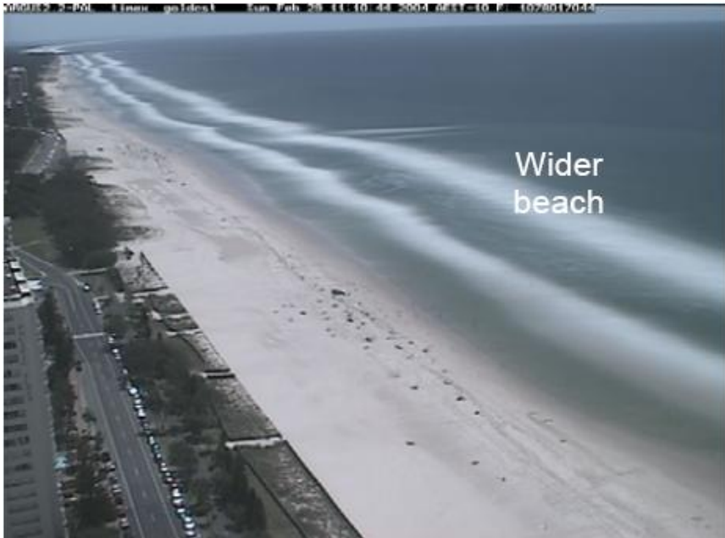
Figure 3.4 Time-averaged WRL image prior to March storm [29/2/2004], demonstrates how successful the Narrowneck submerged reef has been at retaining nourishment material on Surfer's Paradise Beach. (Jackson et al. , 2004)
