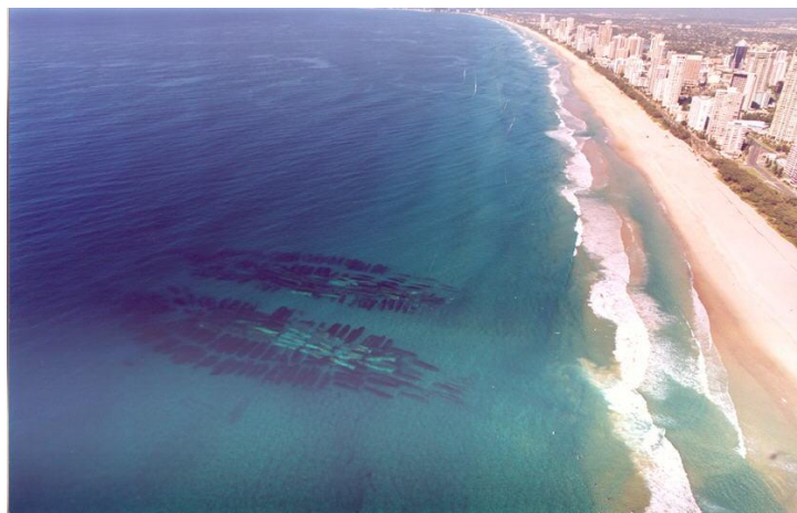
Figure 3.3 The view of Surfer's Paradise with the multi-purpose reef in the foreground (Mead et al. , 2006).
