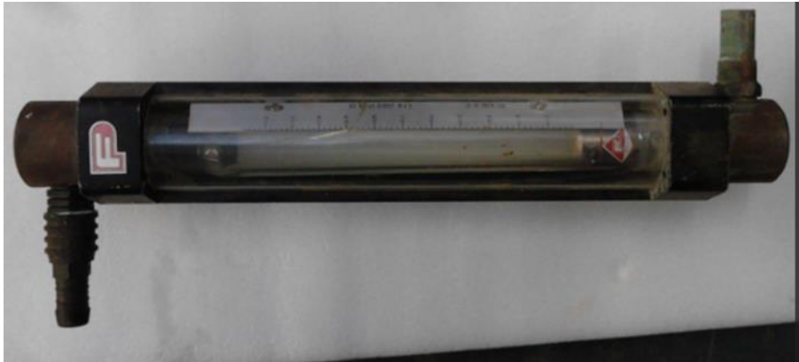
Figure 3.4 Cooling water flow meter
