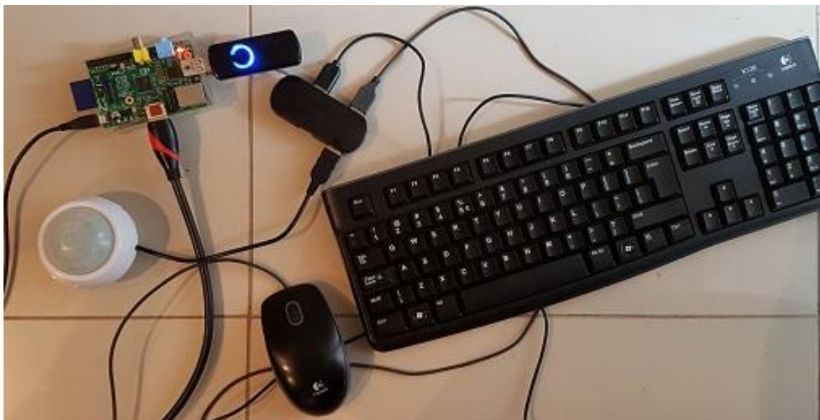
Figure 4-18 Setting up the Z-Wave network and the Raspberry Pi
