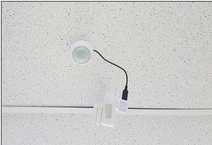
Figure 5-4 Aeotec 4-in-1 sensor mounted onto the ceiling of the laboratory
