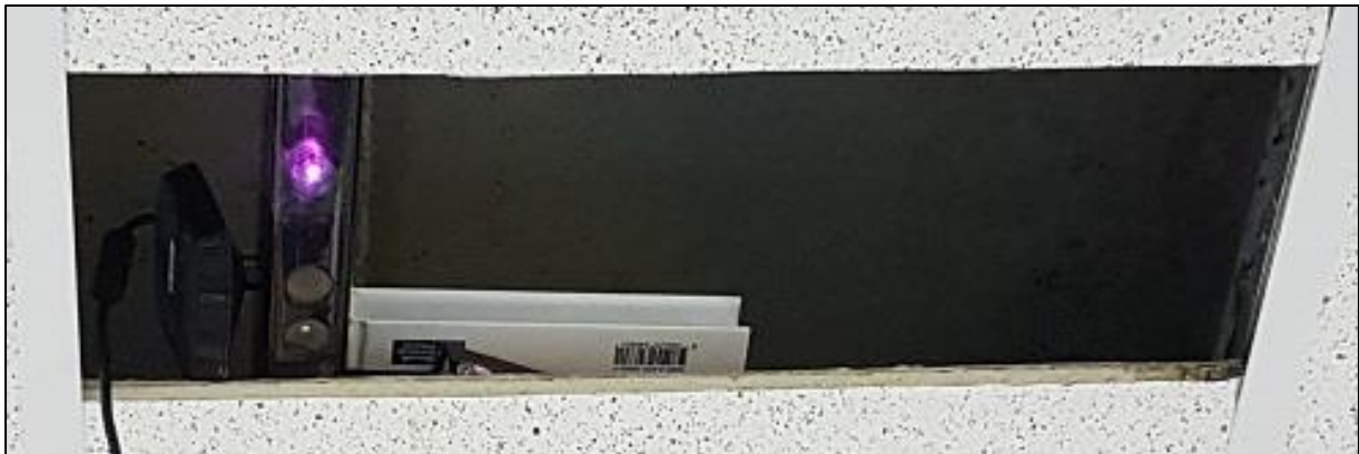
Figure 4-32 Microsoft Kinect mounted on the ceiling
