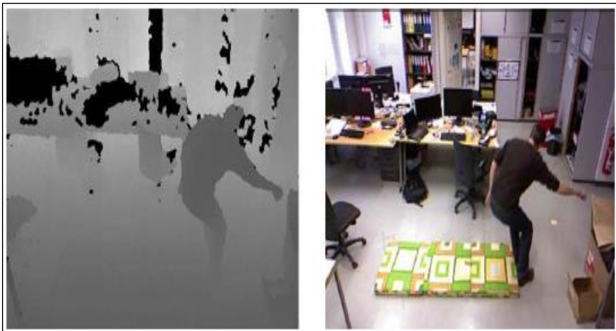
Figure 3-14 Depth buffer image and the corresponding RGB picture
