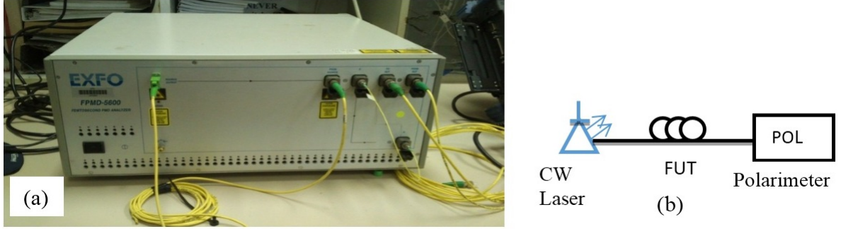
Figure 4.3: (a) Picture of a Femtosecond PMD analyzer (EXFO FPMD 5600) used in the measurement (b) Research set-up used to study the polarization effects. CW is continuous wave and FUT is fibre under test.
