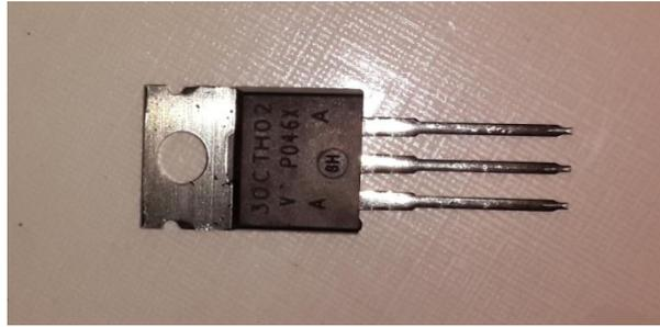
Figure 4-7: Selected rectifying diode D<sub>r</sub> for the MPPT power circuit
