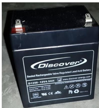
Figure 3-6: Selected lead-acid battery for main energy storage of solar vehicle
