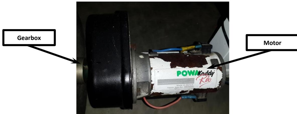
**Figure 3-8: Gearbox assembly and motor of the electric golf trolley**
