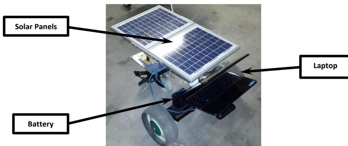
**Figure 3-9: Solar panels mounted on the solar vehicle**
