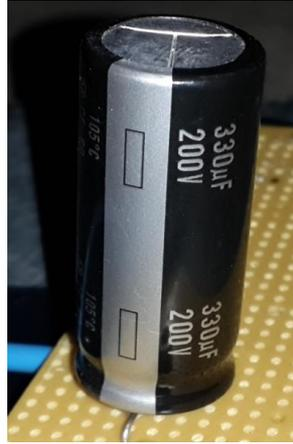
**Figure 4-5: Selected capacitor  $C_{out}$  for the MPPT power circuit**
