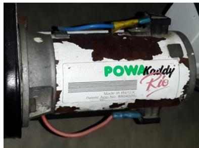
**Figure 3-7: Electric motor selected for the solar vehicle model**
