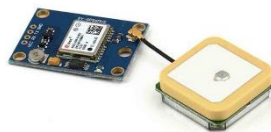
Figure 3-17 NEO-6M GPS (Source: (Anon., 2018))
