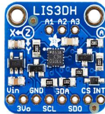
Figure 3-15 LIS3DH (Source: (Anon., 2018))
