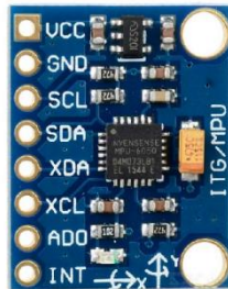
Figure 3-13 MPU-6050 (Source: (Anon., 2018))
