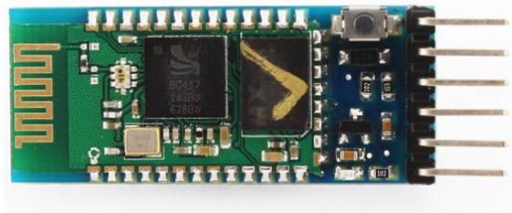
Figure 6-2 Bluetooth Module (Source: (Anon., 2018))
