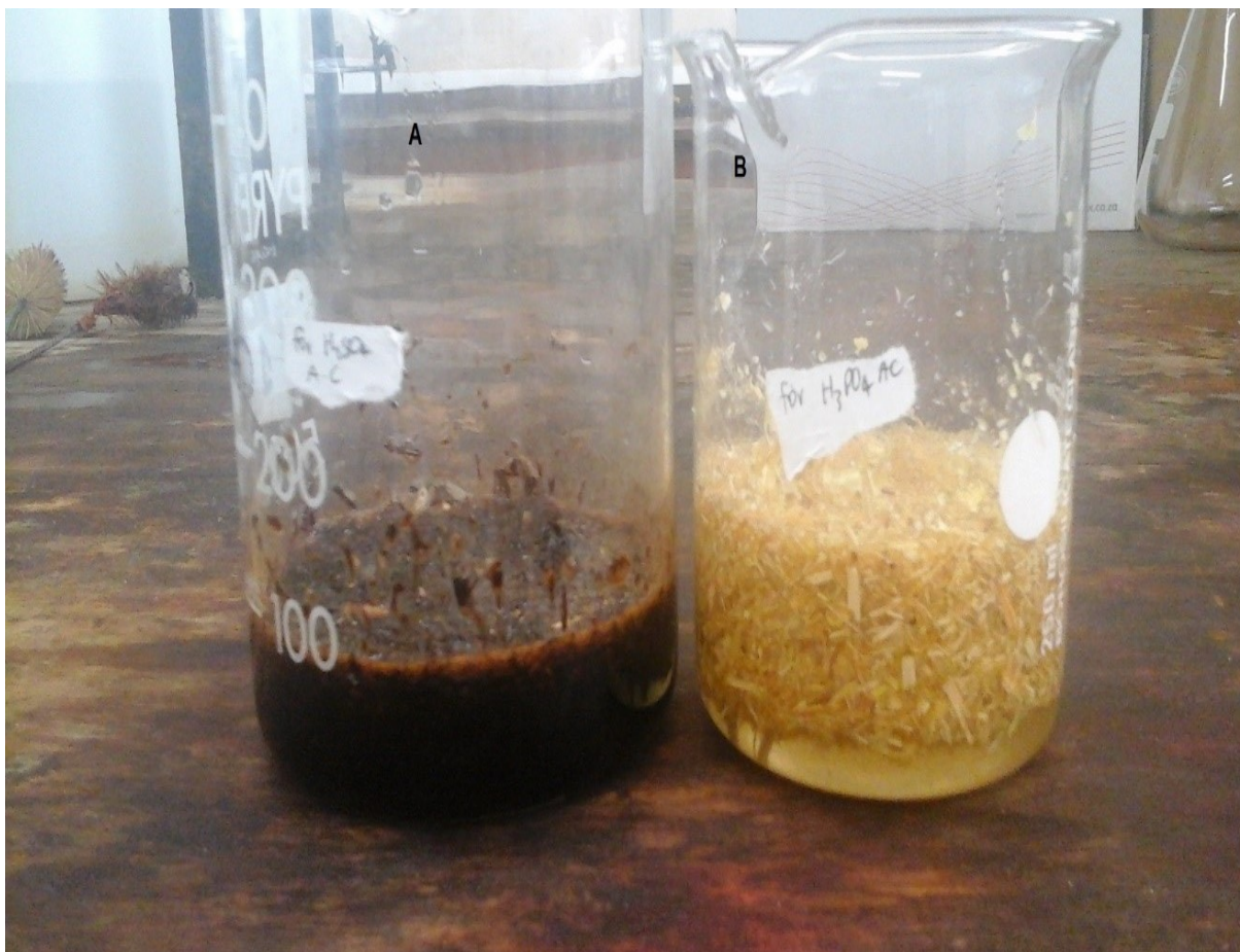
Figure 2.1: The impregnation mixture of Zea mays stem with \text{H}_2\text{SO}_4 (A) and \text{H}_3\text{PO}_4 (B)
