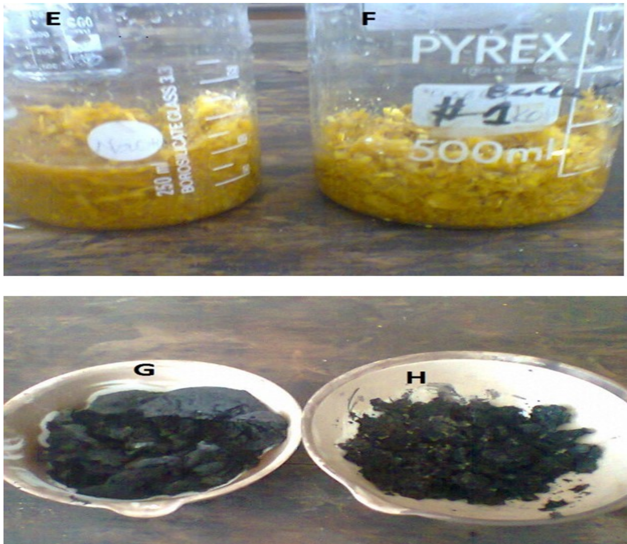
Figure 2.4: Impregnation mixture of Zea mays stem with NaOH (E), KOH (F), and resultant activated carbon from NaOH (G) and KOH (H).
