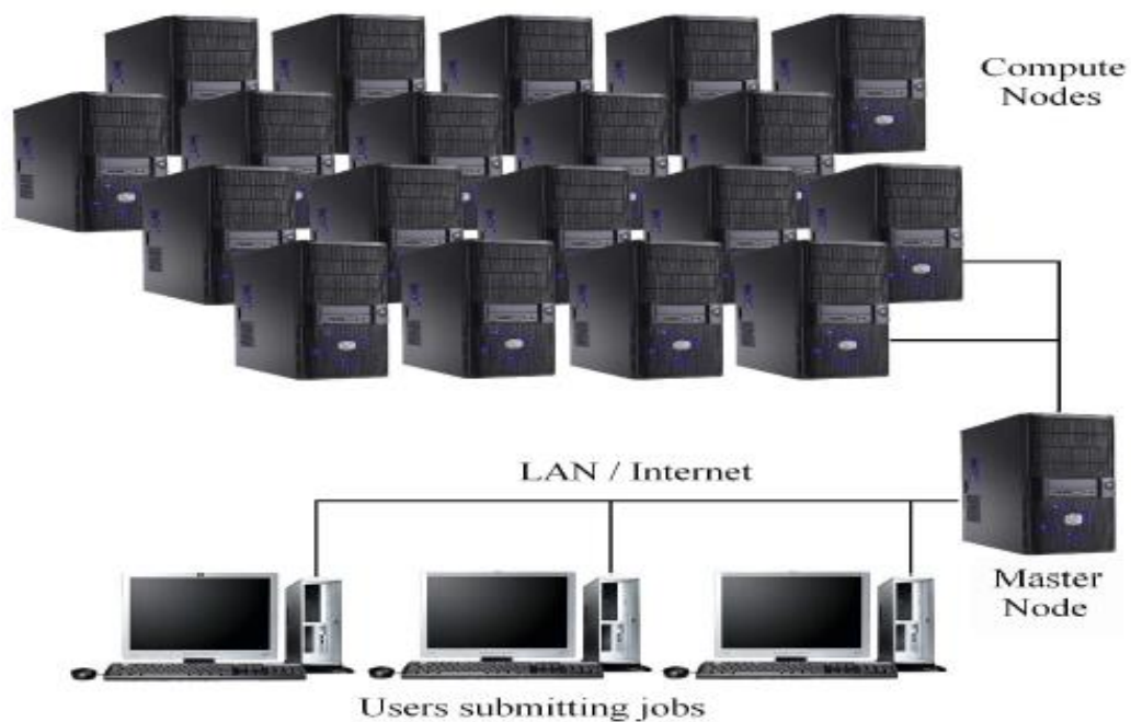
Figure 3.1: High Level Beowulf Architecture (Chavan, 2012).
