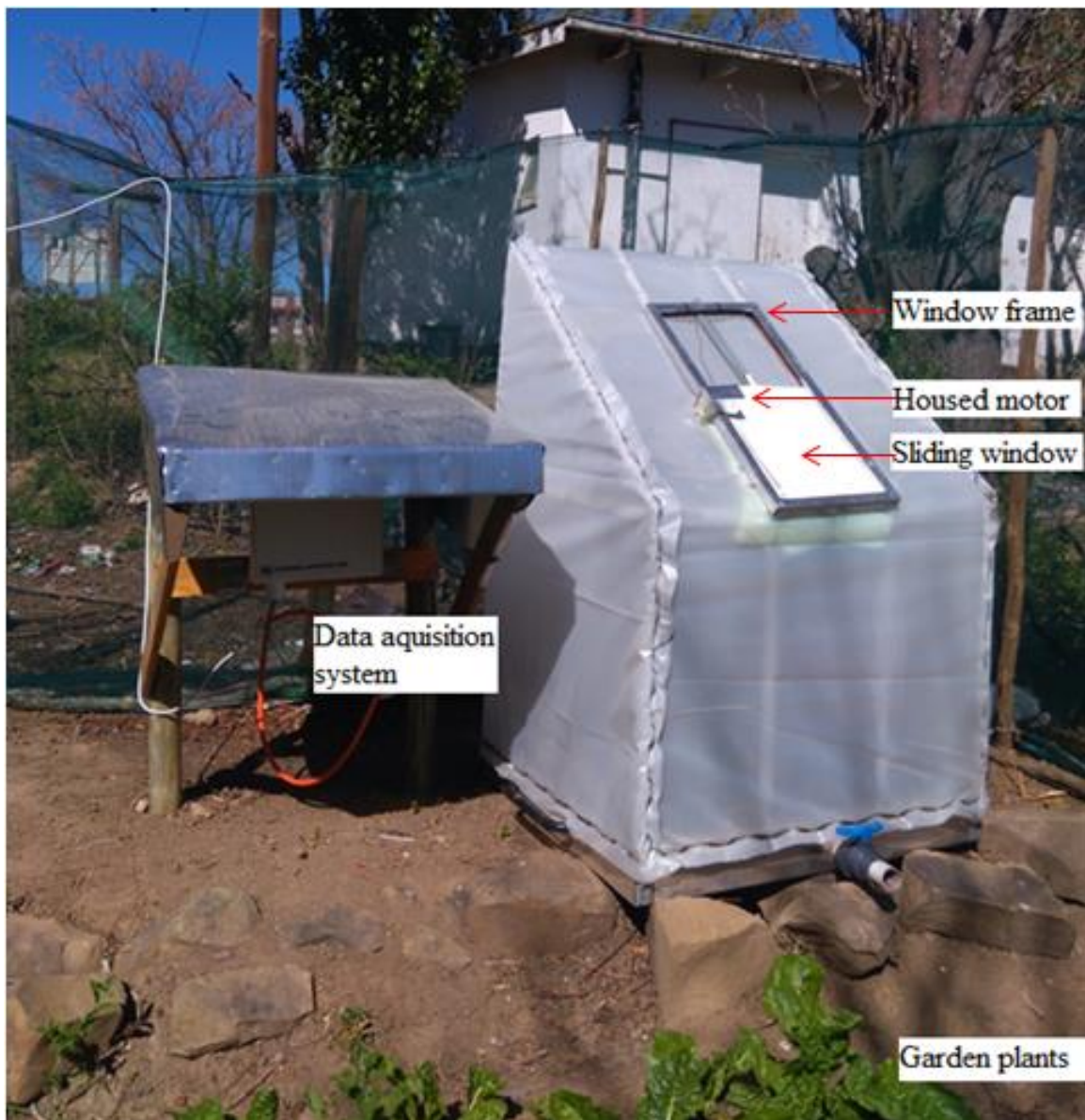
Figure 4.22: Greenhouse regulated temperature biogas digester
