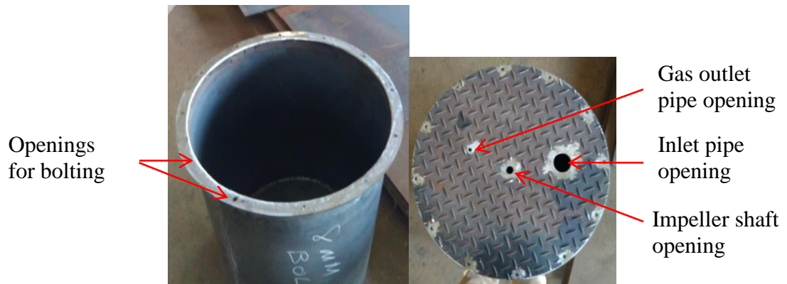
Figure 4.9: Fabricated digester vessel (left) and top (right)
