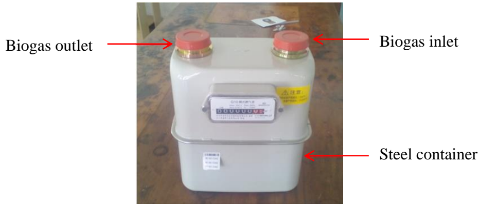
Figure 3.11: Serial residential (SR) diaphragm biogas flow meter
