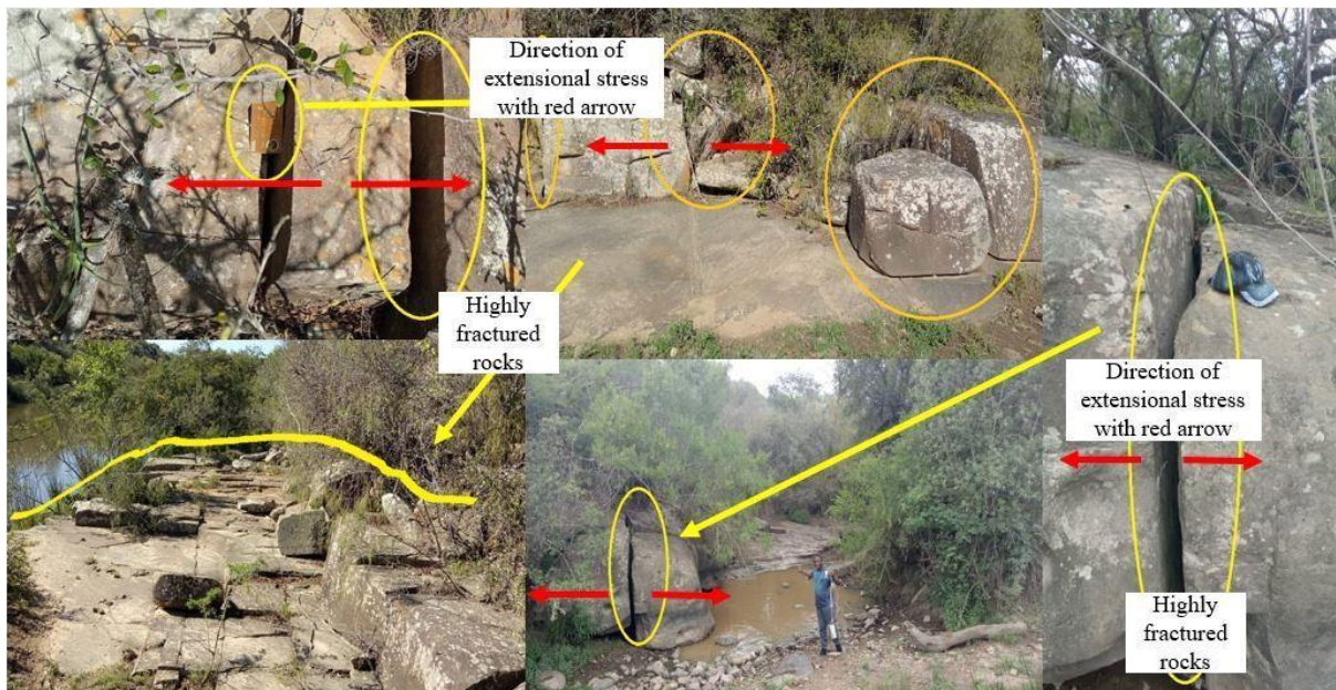
Figure 7. 3: Massive joints in rocks along embankments and channels of the Quencwe River. The direction of joints indicating the effect of extensional stress was indicated with a red arrow. The extensional stress is significant for its productive influence on interflow and recharge from baseflow.
