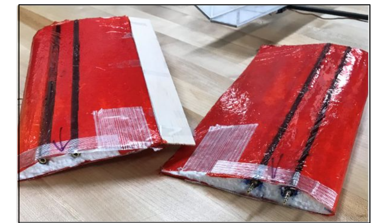
Figure 5 - View of the wing sections from above, including the headphone jacks, spars, and aileron.
