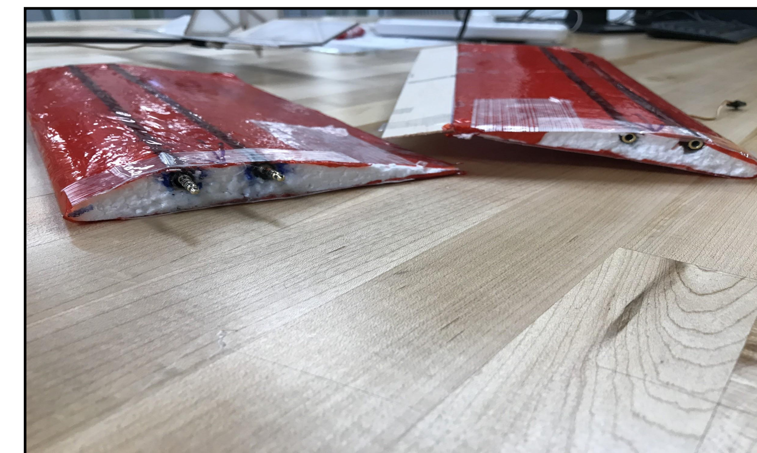
Figure 4 - Cutoff area of the wing with headphone jack connections.
