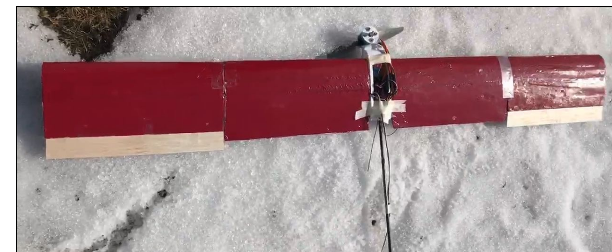
Figure 6– Plane with front of fuselage broken off after flight testing.
