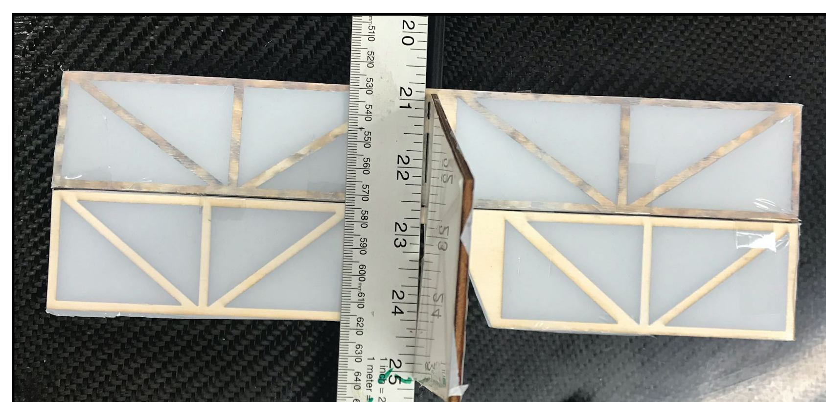
Figure 2 - Overhead view of the tail, displaying the horizontal stabilizer and elevator.
