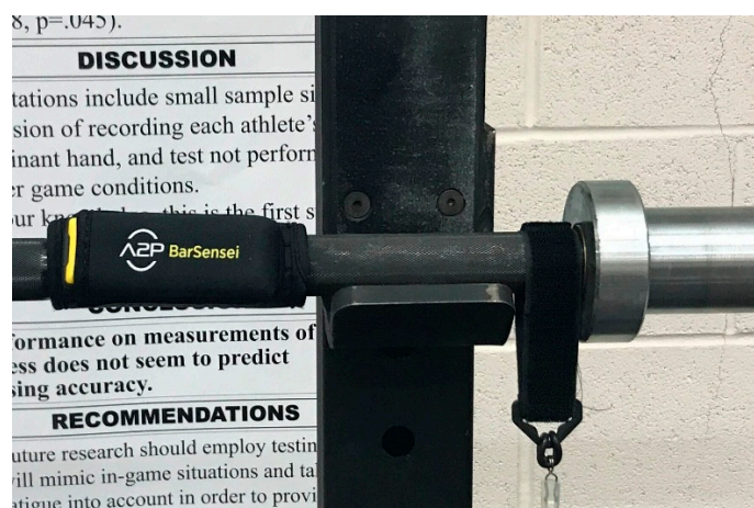
Figure 1. Placement of Bar Sensei and GymAware on a barbell.
