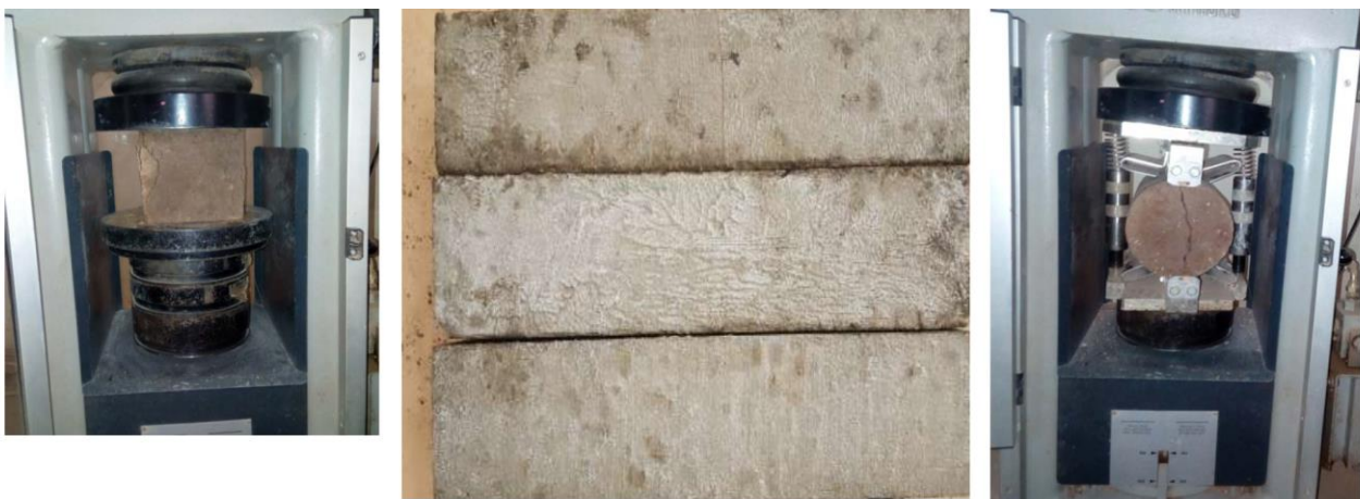
Figure 3- Specimen subjected to Compressive Strength Test, Flexural Strength Test and Tensile Strength Test
