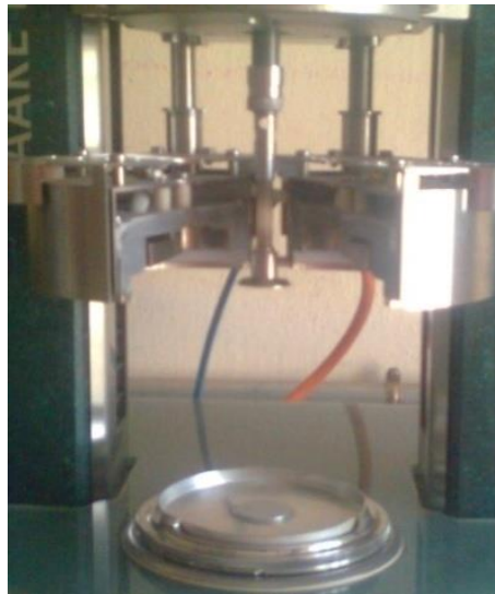
Fig. 1 – Rheometer Haake Rheostress 1 test
