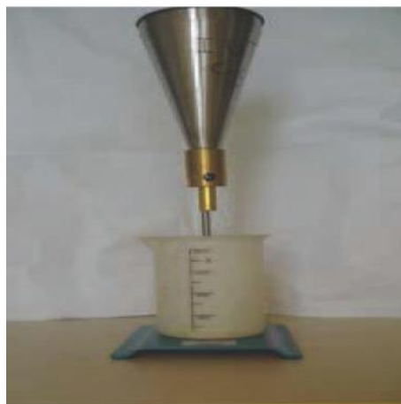
Fig. 2 – Marsh cone test
