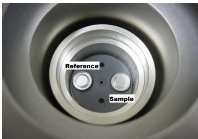
Figure 4.1 Top view of specimen placed on the heat flux Sensor [20]
