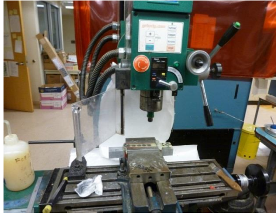
Figure 3.3 Drilling machine used to cut AS4/3501-6 composite laminate
