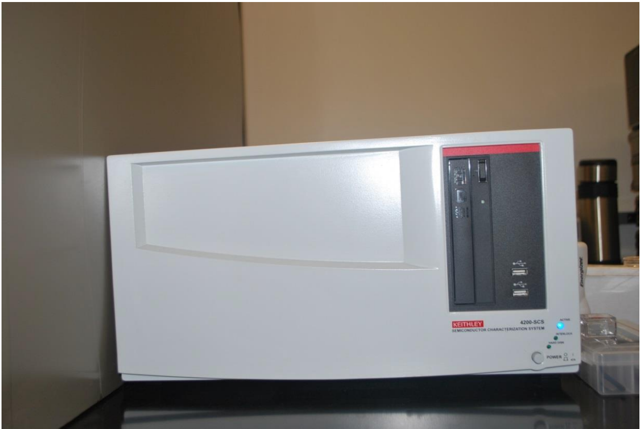
Figure 12. Keithley 4200-S system used for current-voltage measurements.
