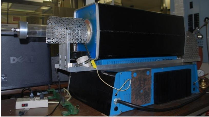
Figure 7. Annealing furnace system.
