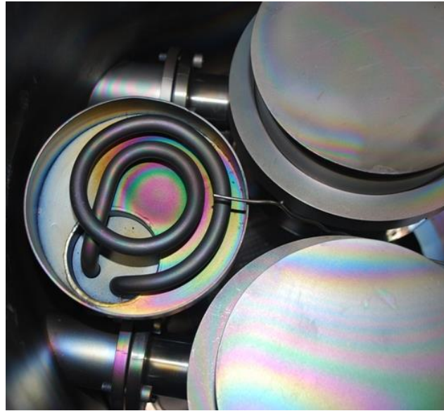
Figure 6. Radiant heater used for ET deposition.
