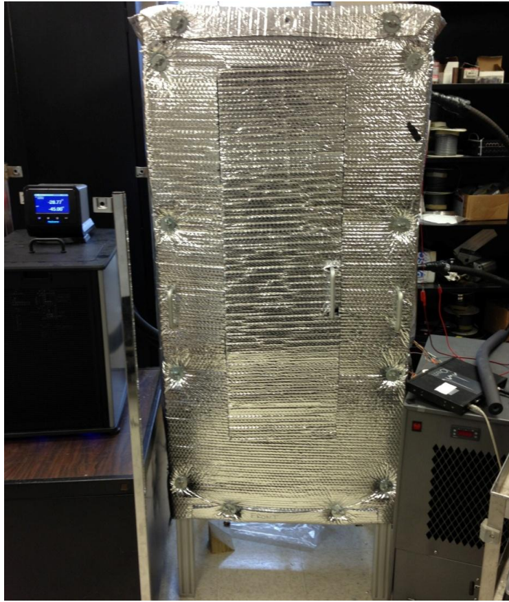
Figure 24. Environmental chamber used to simulate subcooled conditions.
