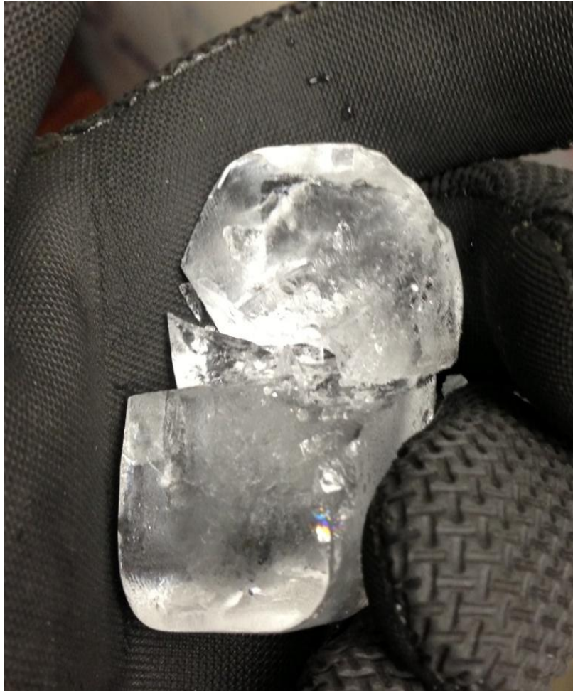
Figure 23. Ice cracked due to the application of cyclic loading.
