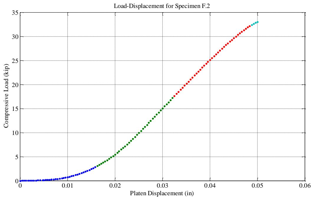
Figure Load-Displacement Curve for F.2
