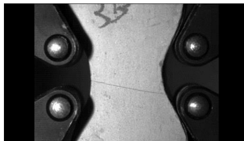
Figure 4.25. View of Briquette F.3 with the Crack Propagated through the Briquette
