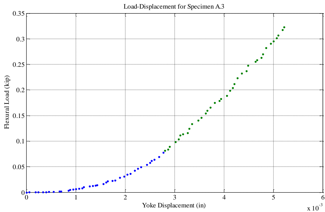
Figure Load-Displacement Curve for A.3
