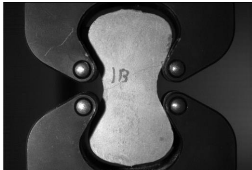
Figure 4.19. View of Briquette F.1 with the Crack Propagated through the Briquette
