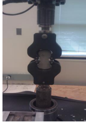
Figure 4.15. Test Set Up for the Direct Tension Test
