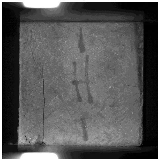
Figure 4.7. Failure Pattern of Cubical Specimen B.2
