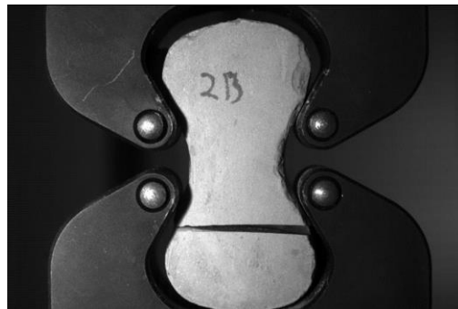
Figure 4.23. View of Briquette F.2 at the End of the Test
