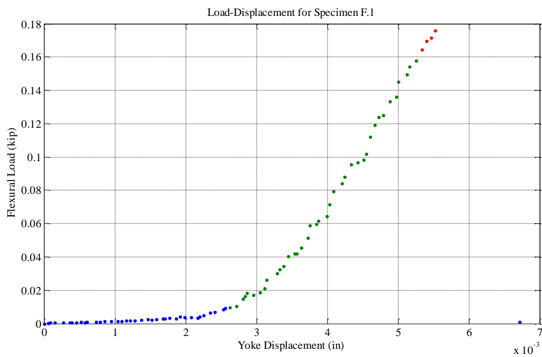
Figure Load-Displacement Curve for F.1
