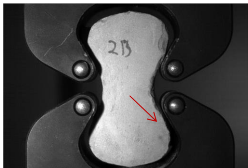
Figure 4.21. View of Briquette F.2 at the Initiation of Failure
