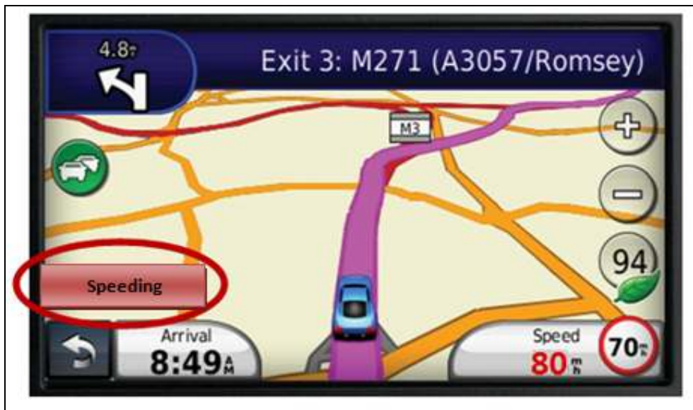
Figure 3.6. GPS Speed Alerting Features.
