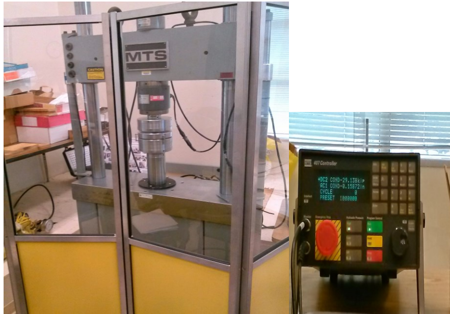
Figure 13. MTS 810 compression test with 407 digital controller.
