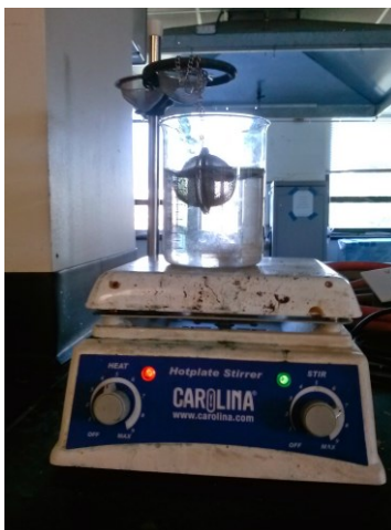
Figure 8. Hotplate stirrer with magnetic field
