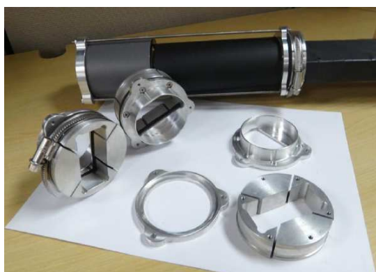
Figure 4.3: Quartz bar-PMT connector brace
