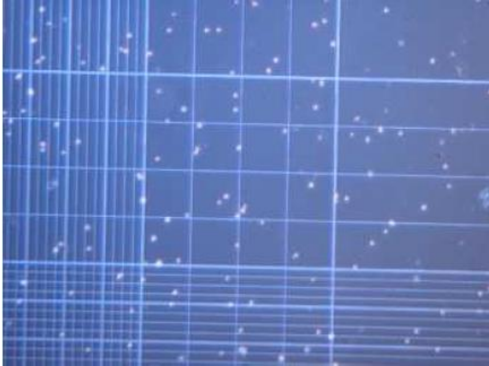
Figure 10. Cell counting procedure using hemocytometer
